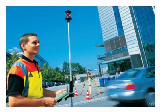
How practical when you can measure from the target point! With RCS you can record information and perform surveying tasks on your own.
